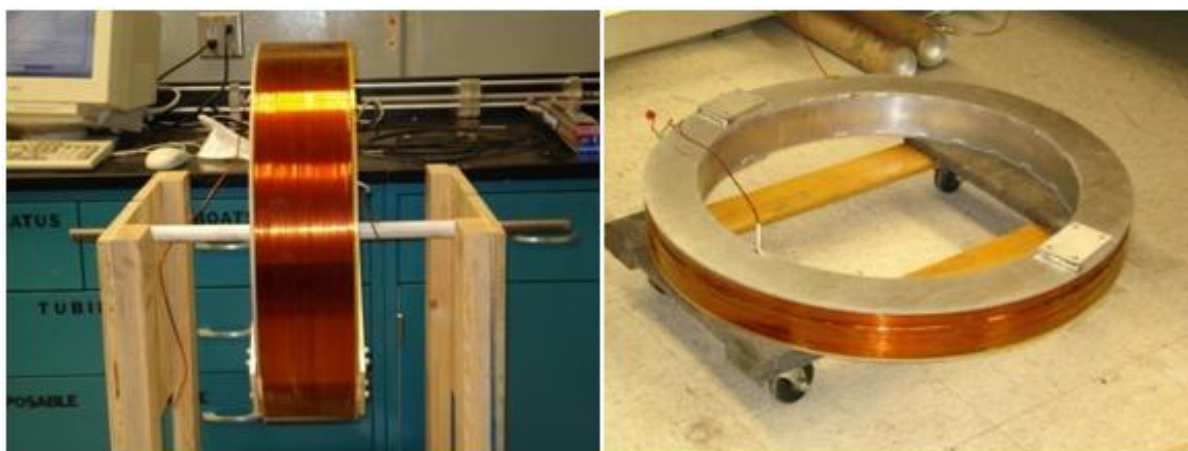
Fig. 2.31. Image of the coils used for the first positron beam switchyard.
