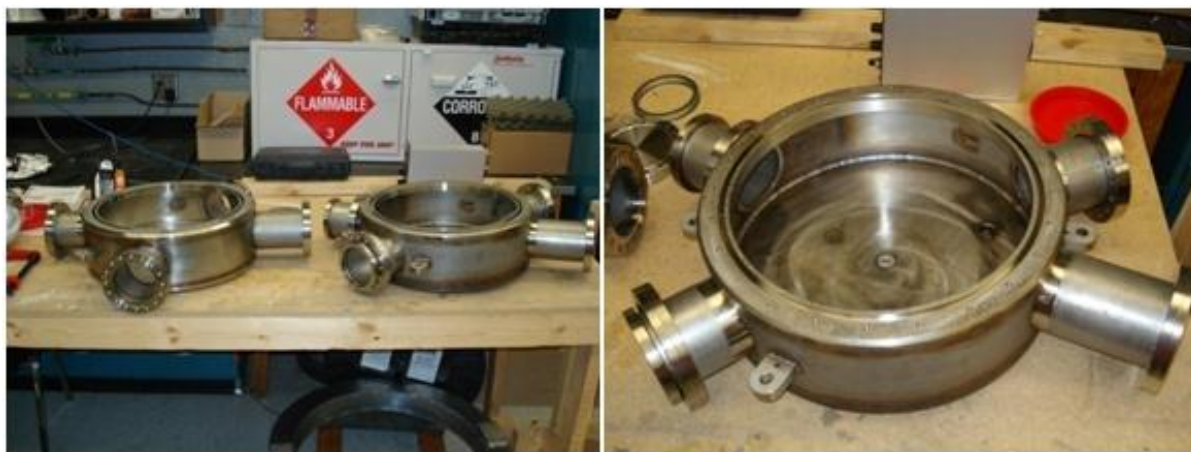
Fig. 2.25. Images of the vacuum chambers for the two positron beam switchyards.
