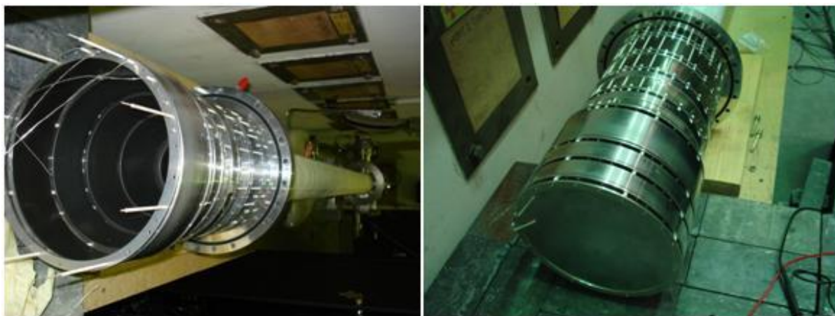
Fig. 2.23. Images of the slow positron extraction optics with (right) and without (left) the moderators installed.
