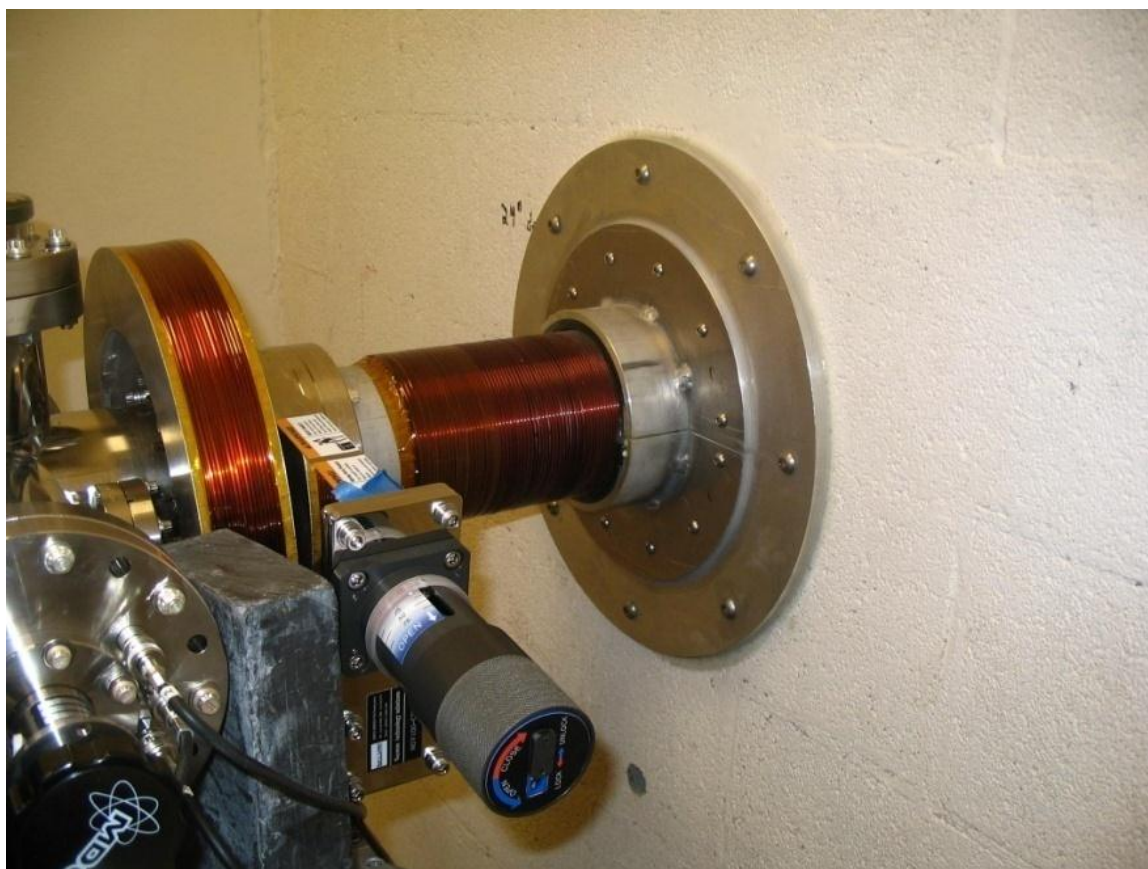
Fig. 3.11. Image of the solenoid penetrating the shielding walls into the e^+ -PALS spectrometer lab with the accompanying gate valve.
