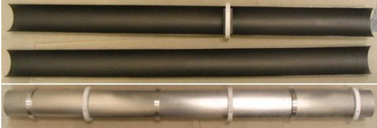
Fig. 4.17. Image of the drift lens for the pulsed positron spectrometer. The lens is cut in half and reassembled to allow the application of graphite to the internal surface and the installation of the internal shield.
