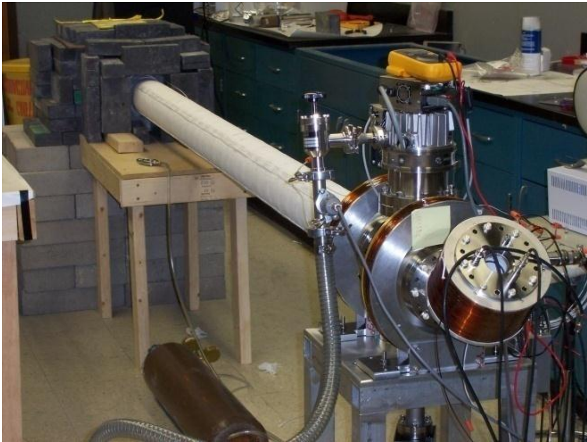
Fig. 3.1. Image of the intense slow positron beam while undergoing bench top testing.
