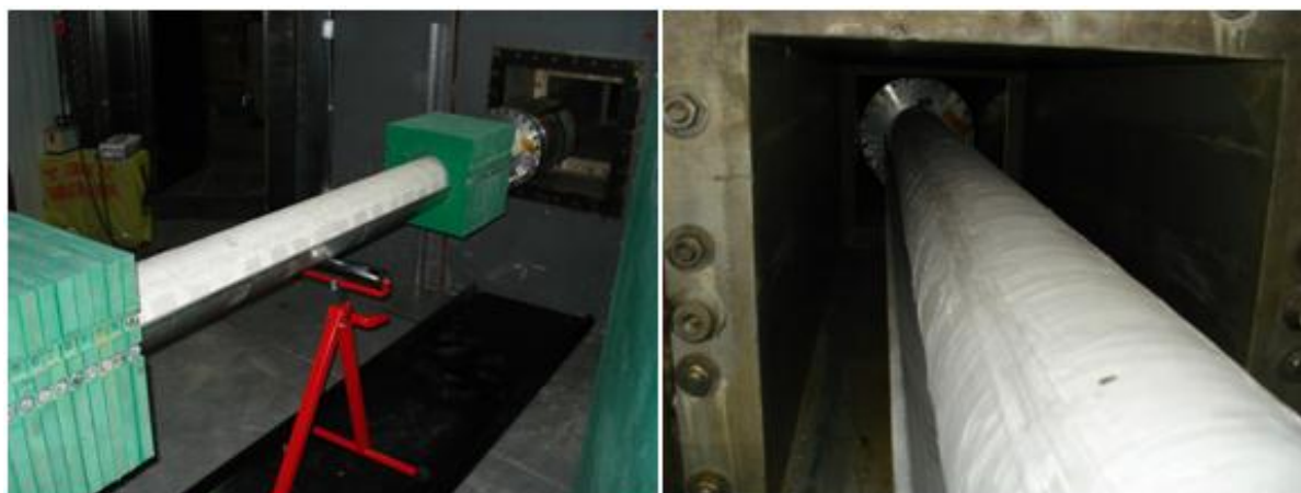
Fig. 3.8. Images of insertion of the slow positron beam into beam tube 6.
