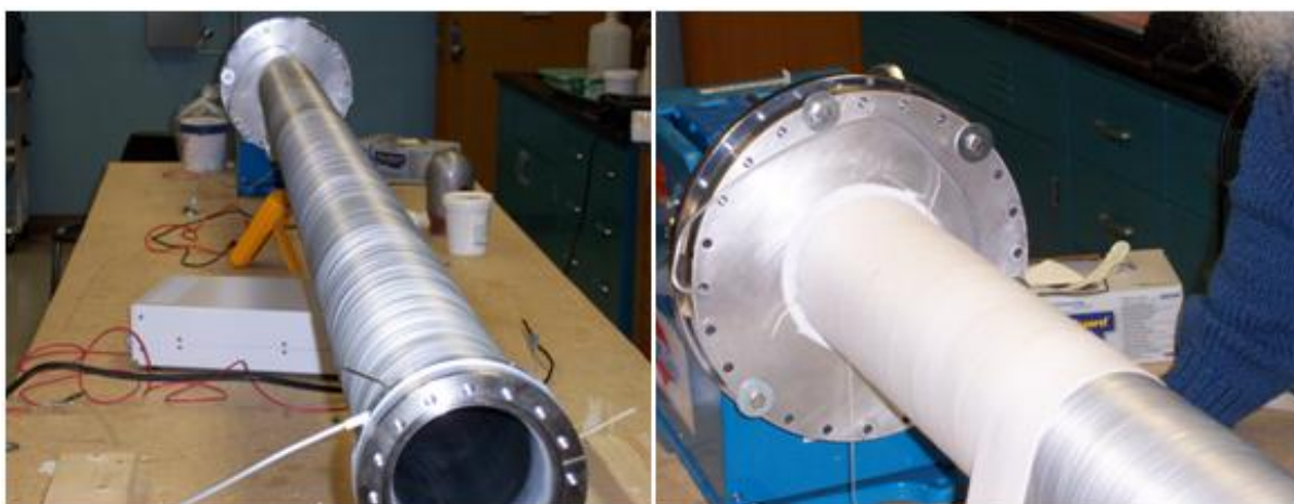
Fig. 2.28. Images taken during the winding of the main solenoid of the slow positron beam.
